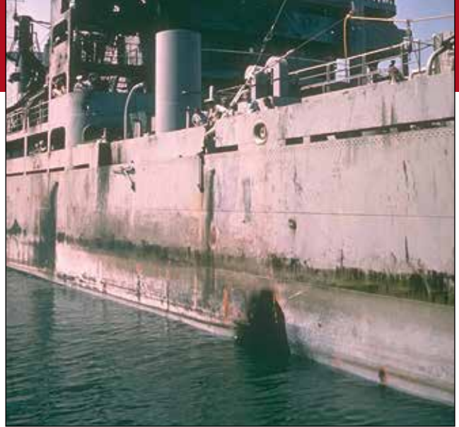
The torpedo hit Liberty at and below the waterline, creating a 24- by 39-foot hole in her hull.
