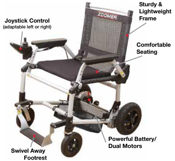
aluminum frame makes it durable and comfortable. It's dual motors power it at up to 3.7 miles per hour
