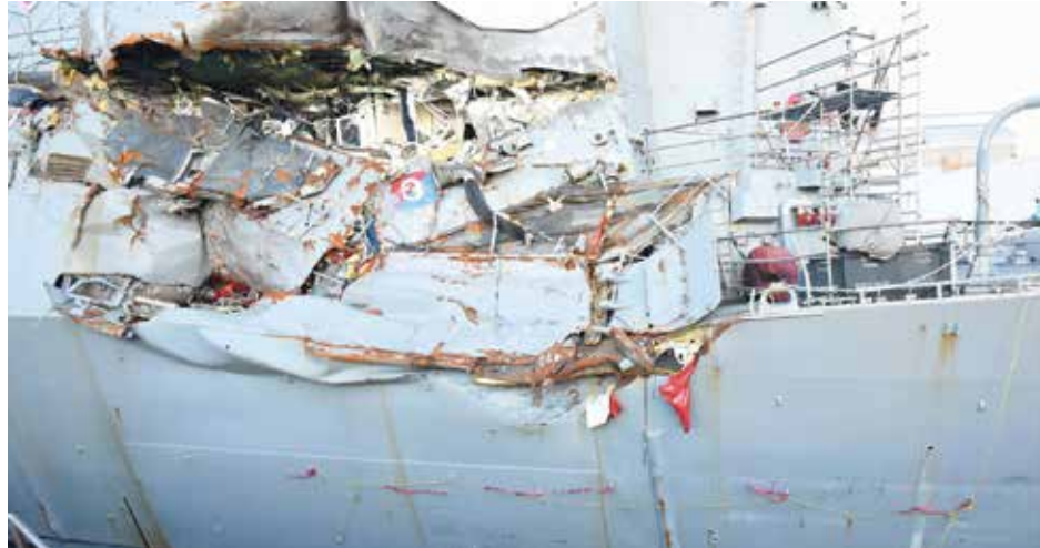
The Arleigh Burke-class guided-missile destroyer USS FITZGERALD (DDG-62) sits in Dry Dock 4 at Fleet Activities in Yokosuka for repairs sustained from its June 17 collision with a merchant vessel. U.S. Navy photo by MC1 Leonard Adams
