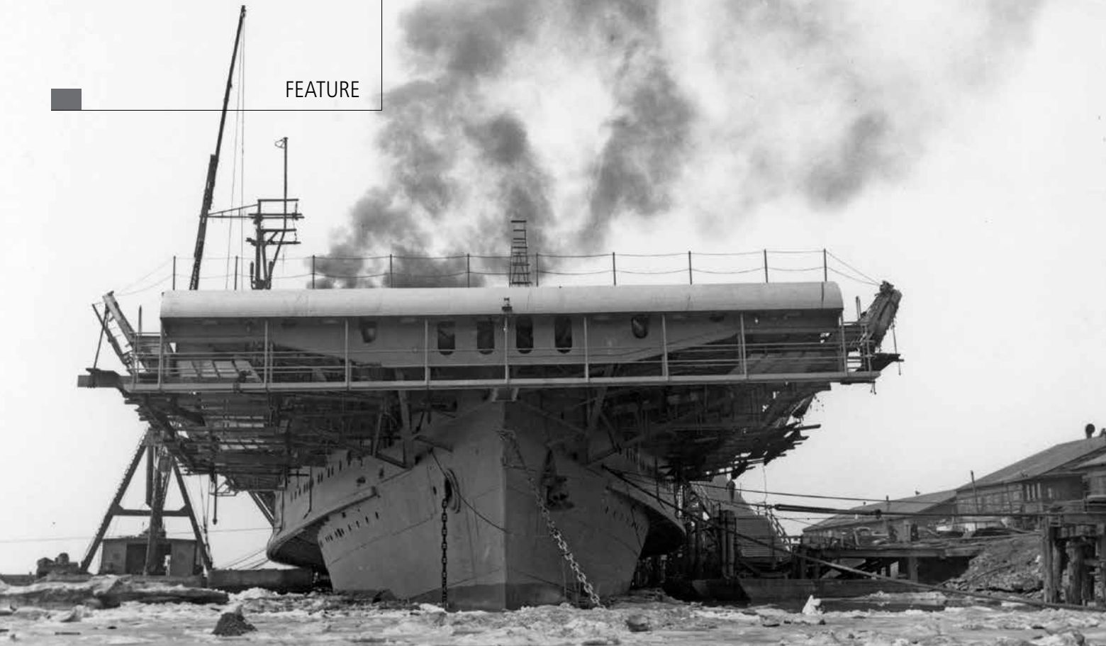
The USS SABLE (IX-81) moored in an icy harbor in 1943. Note the steam exhausting amidships. The location may be Buffalo, New York, where it was converted from the side-wheel excursion steamship Greater Buffalo . Official U.S. Navy photograph, now in the collections of the National Archives.
