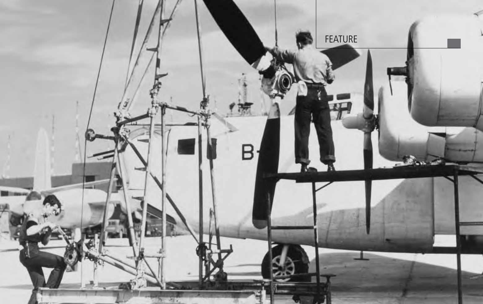
A Consolidated PB4Y-1 patrol bomber receives a new propeller while undergoing maintenance at Naval Air Station Norfolk, Virginia, in December 1943. Note the hand-powered crane and the JM-1 target tug in the left background. Photo courtesy of the Naval History and Heritage Command.
