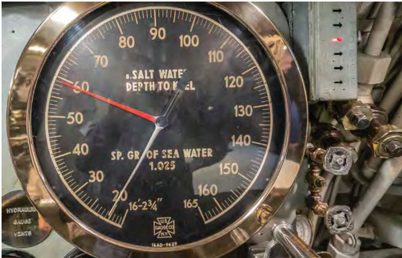
A close-up of a depth gauge on USS BOWFIN . Balao-class submarines like BOWFIN were tested up to a depth of 400 feet. Photo by Klodian.
