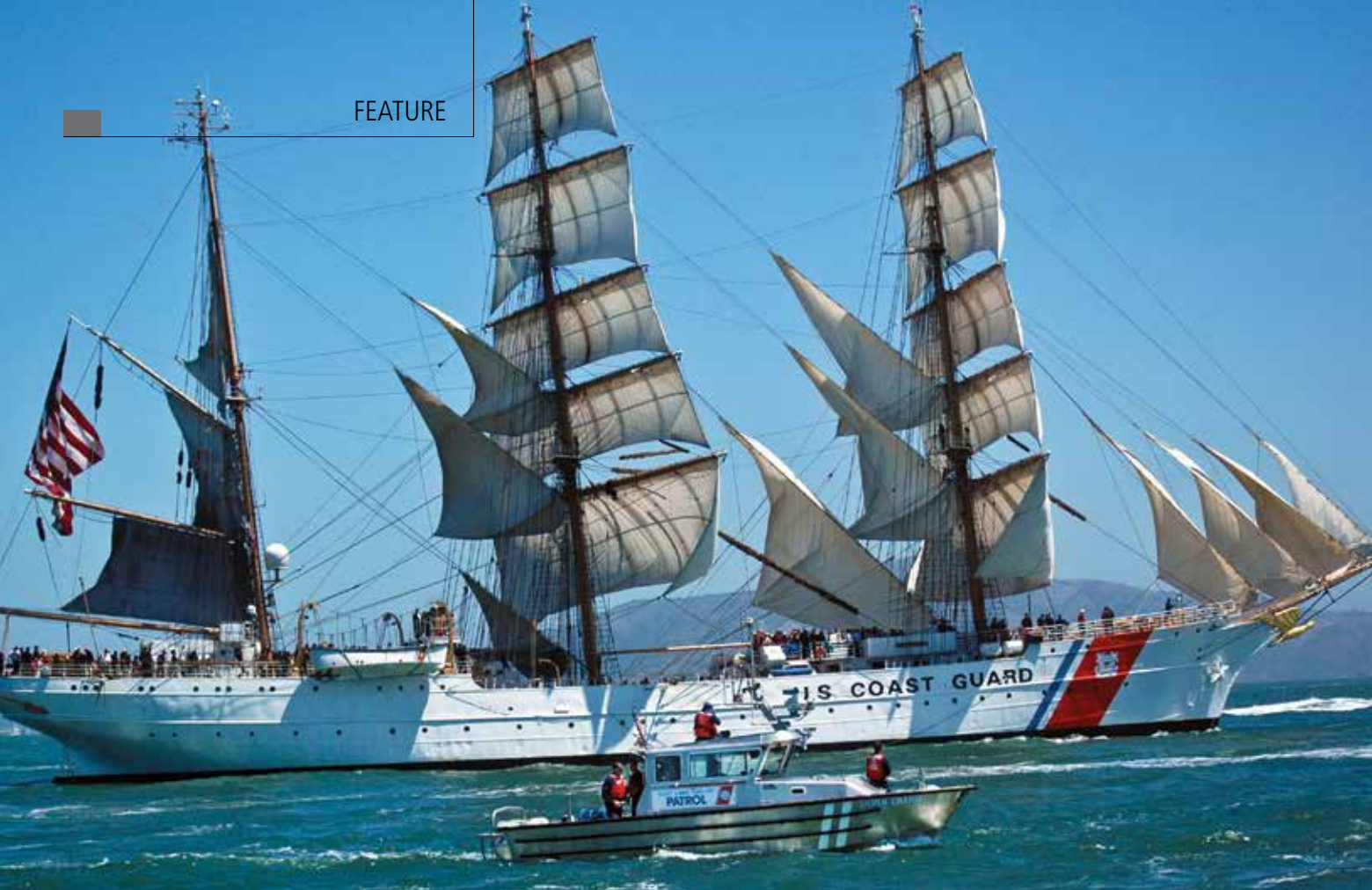
The U.S. Coast Guard Auxiliary Vessel SILVER CHARM escorts Coast Guard Cutter EAGLE , a three-masted sailing barque with 21,350 square feet of sail, during the Festival of Sail parade in San Francisco Bay, on July 23, 2008. The cutter's hull is built of steel four-tenths of an inch thick and has two full-length steel decks with a platform deck below. Commissioned in 1946, the EAGLE is one of the oldest ships in the U.S. Coast Guard fleet. Photo by Eric J. Hebert, USCG Auxiliary.
